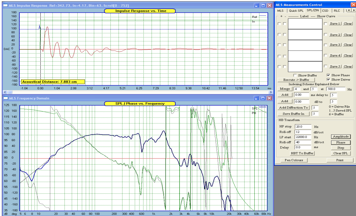
Figure 16.132. Close-mike measurements of a wooferdriver.
