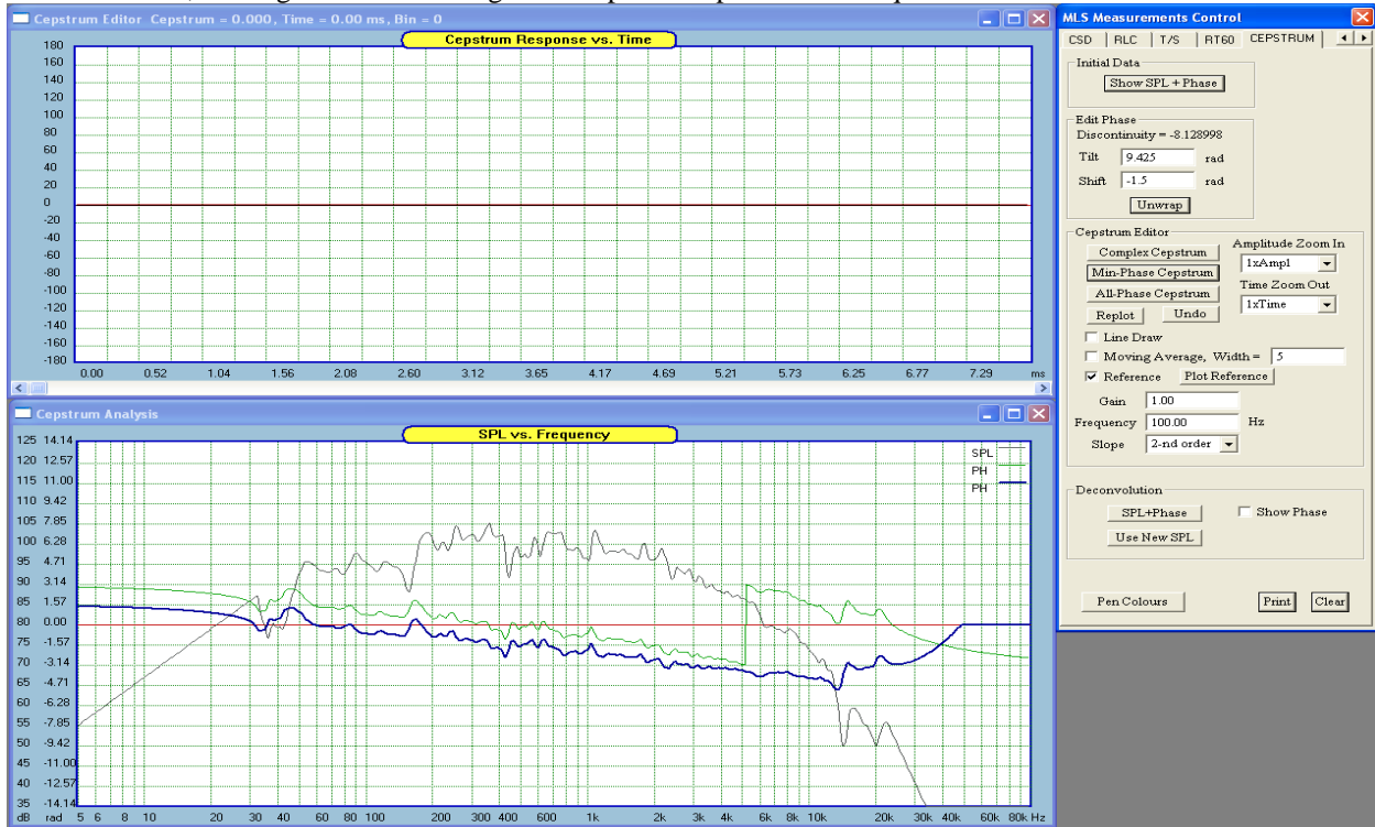
Figure 16.123 “Unwrapped” and adjusted (shift = -1.5) phase response.
