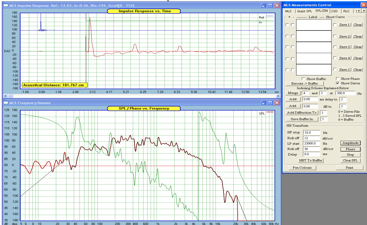
Figure 16.121 HBT (amplitude + phase) of the example midrange driver
