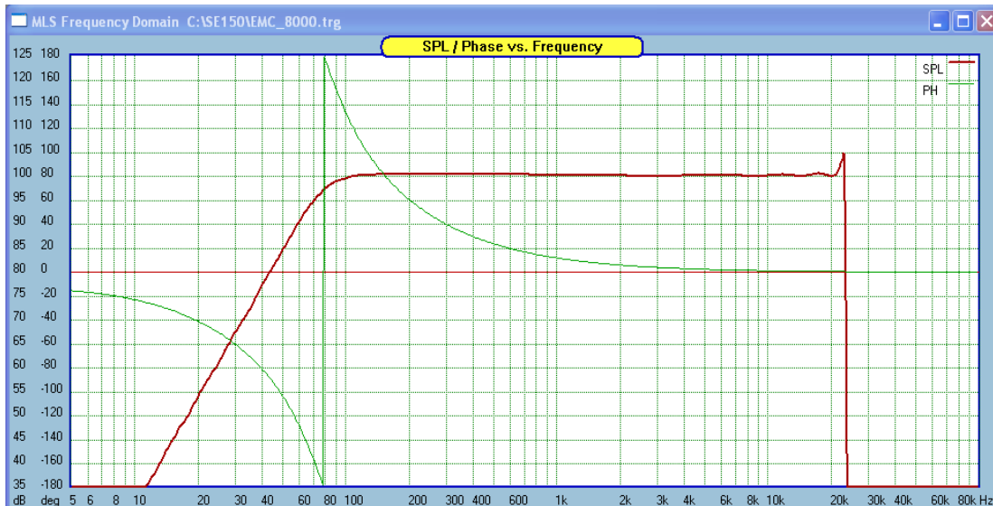
Figure 16.148. Vented (4-th order) loudspeaker system simulated SPL.
