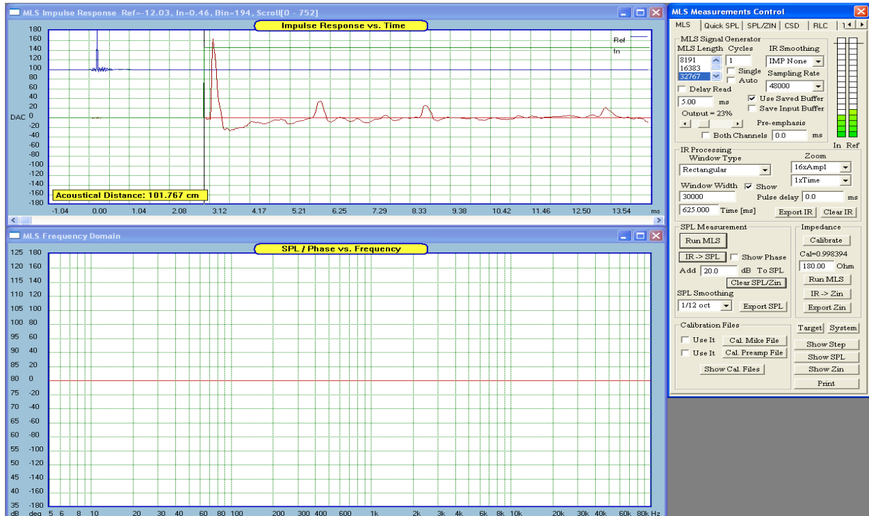
Figure 16.119 Impulse response of an example midrange driver.
