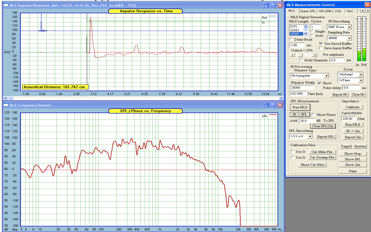
Figure 16.120 SPL of the example midrange driver
