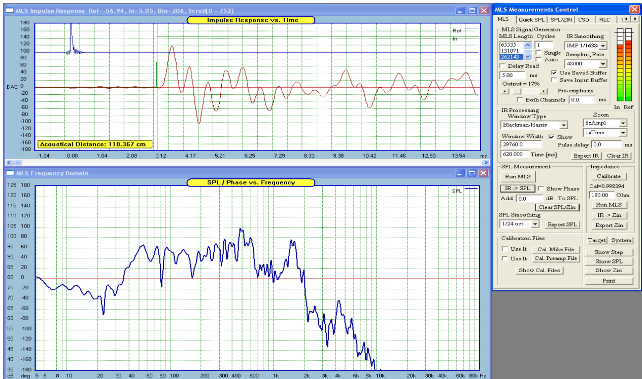
Figure 16.137. The same loudspeaker measured in reverberant environment, with the microphone at appr 1m distance is shown above. The deterioration in SPL curve is very dramatic.
