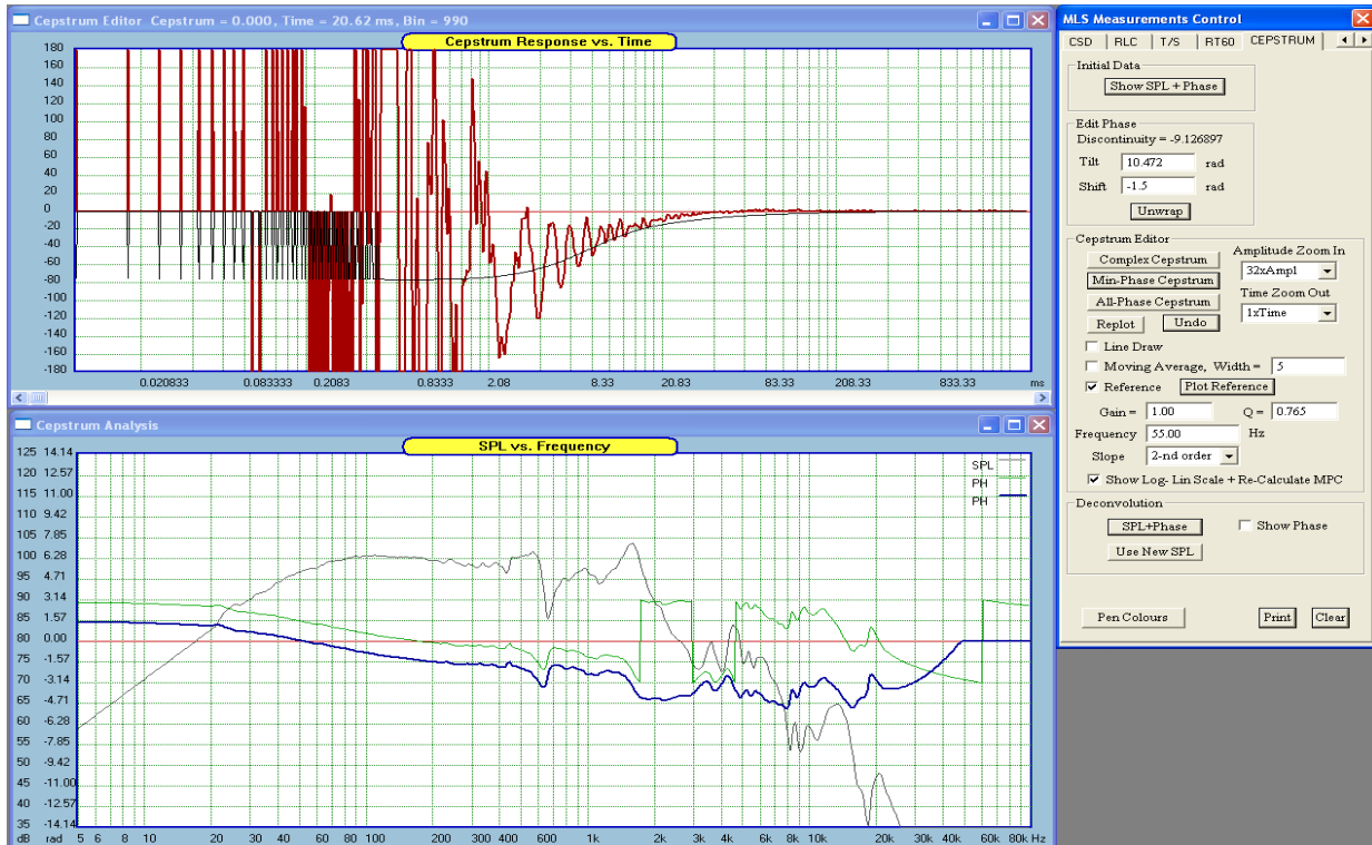
Figure 16.133 Using the log-log scale, coupled with guiding analytical curve, you can see the shape of the tail a lot better. This is where the HBT initial tailing will also manifest itself to some degree.
