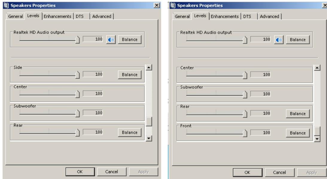
**All other sliders need to be turned down to 0, to avoid signal feed-through.**
