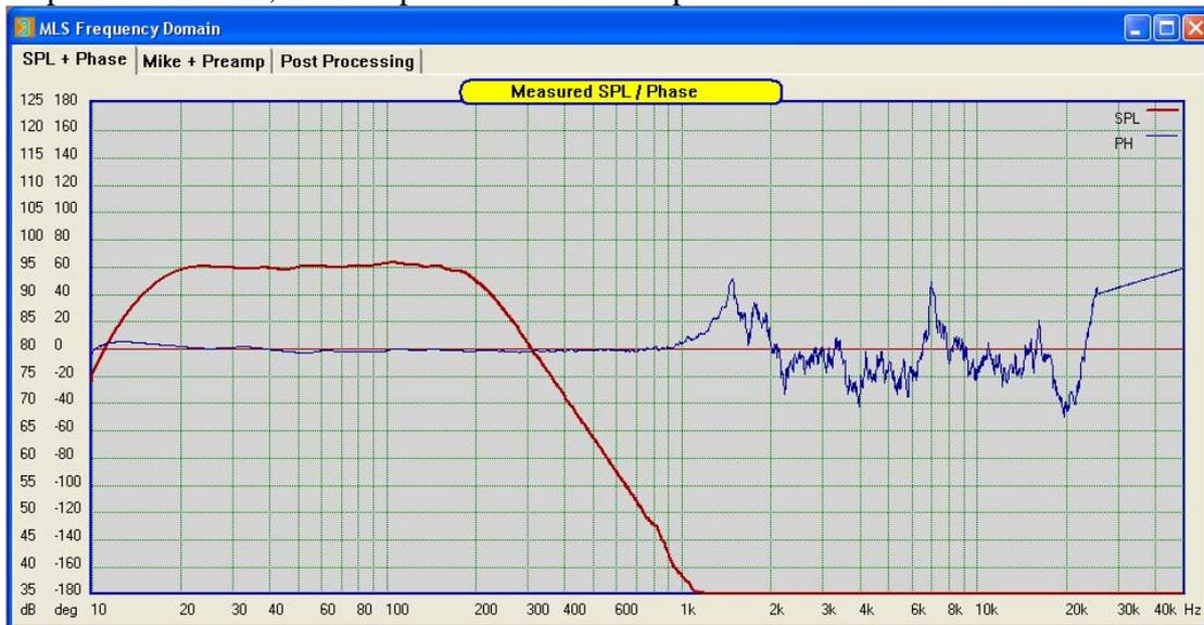
The power of HBT equalization is clearly evident in the final frequency response plot. The SPL / Phase were measured in-room, but still exhibit remarkable flatness and linearity. The same measurement conducted in an anechoic chamber would result in even smoother curves. As shown on the MLS measured plots earlier, I started with clearly sub-optimal, vented enclosure, and turned it to a perfect subwoofer with 3dB bandwidth of 16Hz-200Hz.
