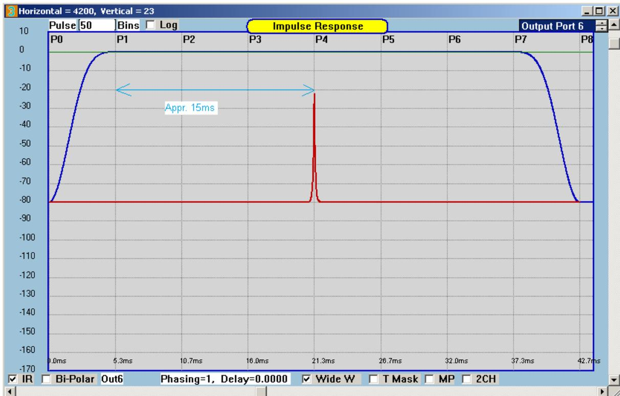
It is observable, that there is no visible ripples on this picture. It does not mean, that there is no pre-ringing – it only means, that pre-ringing is extremely small.
