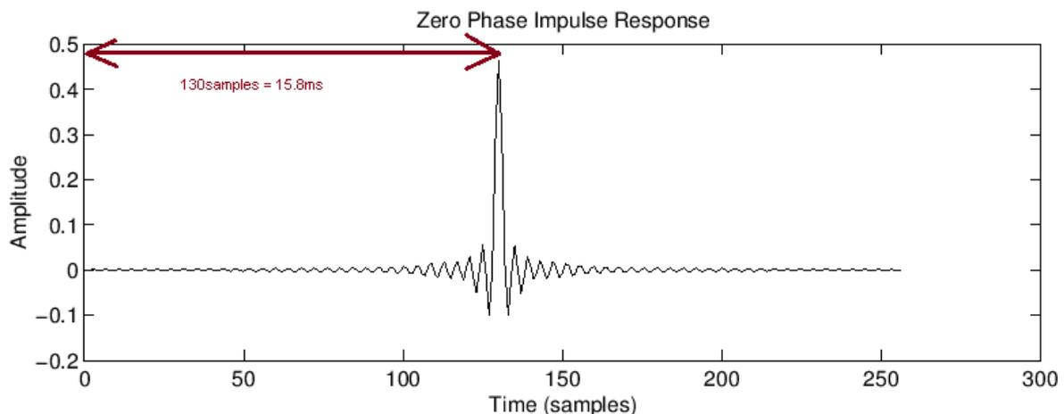
The peak of the impulse response is located at **130samples**, so figures, that **pre-ringing extend over 15.8ms**.
