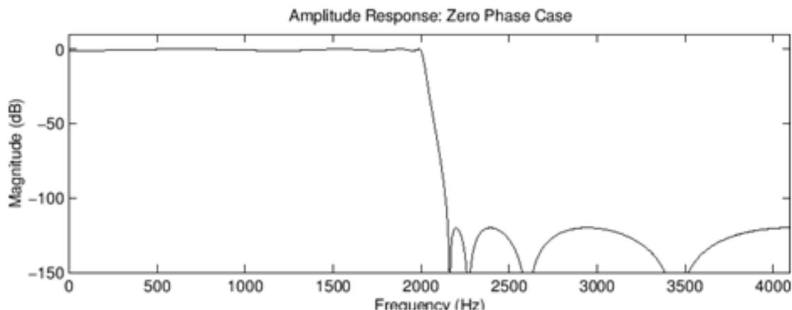
Frequency response is shown above. Sampling rate was  $F_s = 8192$ , so one sample is **0.122ms**.
