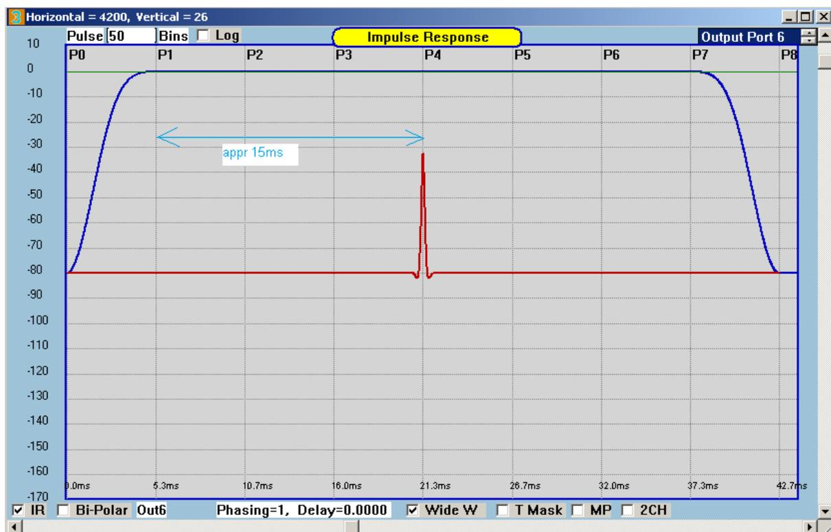
It is observable, that there is only one small ripple, extending to less than 1ms on both side of the peak.
