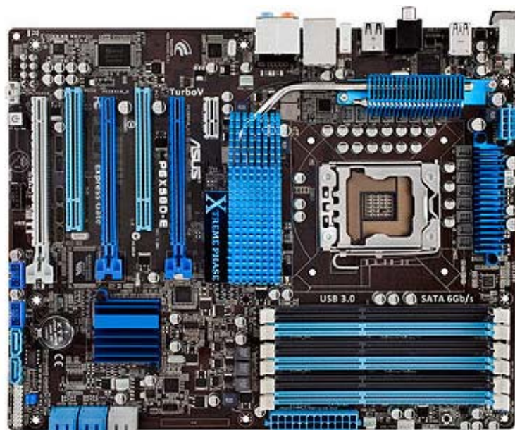
Figure 4. ASUS P6X58D-E motherboard with 2 PCI slots and Realtek® ALC889 8-Channel High Definition Audio CODEC, and coaxial SPDIF output.
