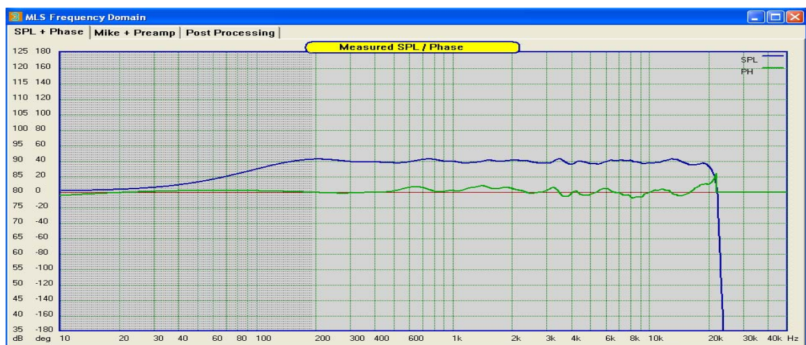
Figure 25. Equalized SPL and phase in 2-way system.
