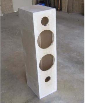
Finally, the exterior is primed and spray-painted with 4 layers of water-based enamel paint. Total construction time was about 10 hours. Fully assembled front loudspeaker is shown below.
