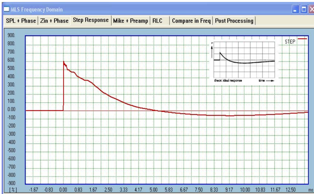
For comparison - Step Response of DSP equalized loudspeaker. Frequency response of this 2-way loudspeaker is also shown on the last page.
