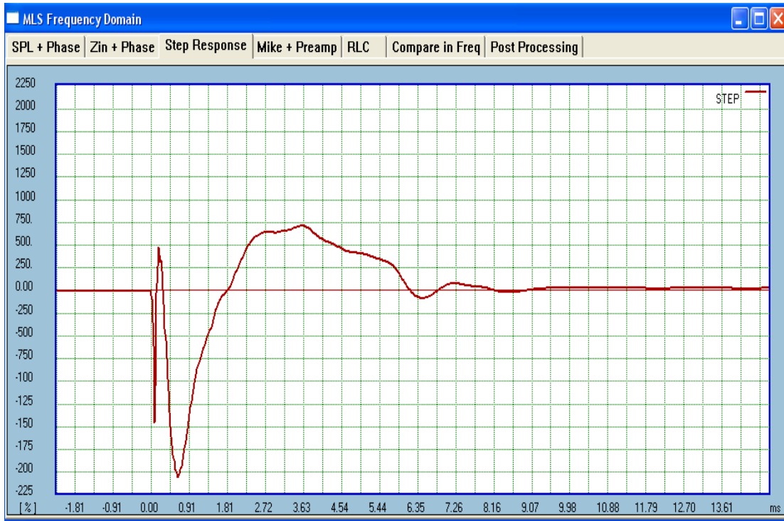
2-way Abbey's Step Response. Maximum output occurs at around 0.60ms after the pulse was applied. Published frequency response of Abbey loudspeaker is shown on the last page of this paper.
