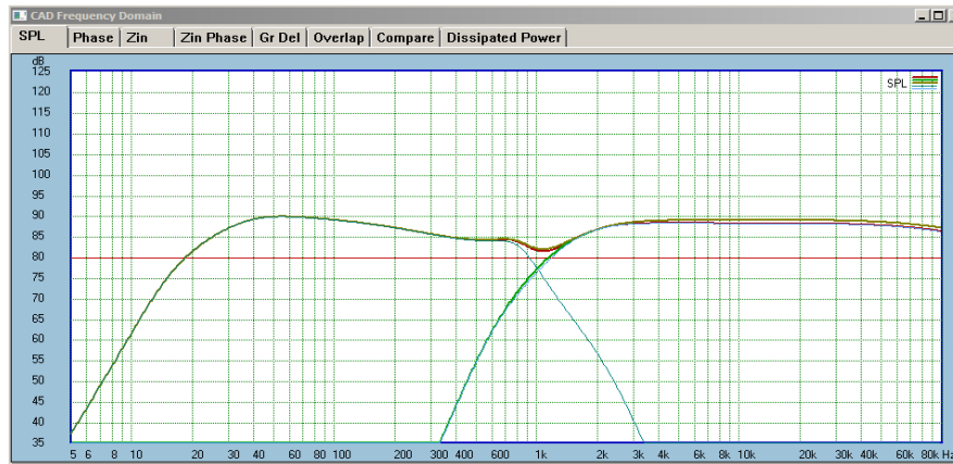
Example of driver files SPL/Zin data created in Enclosure Design screen
