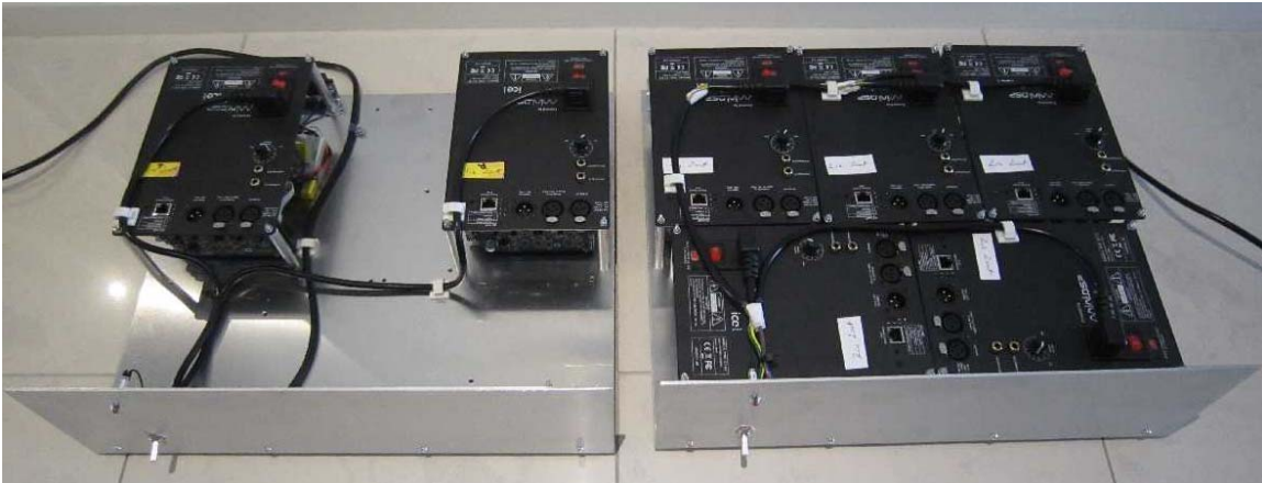
Both amplifiers completed. Left – Subwoofer amplifier, Right – surround channels amp.
