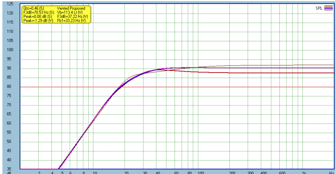
Figure 13. SPL curves of a typical woofer – varying TS parameters.
