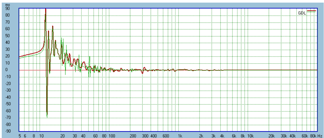
Figure 7. Corresponding GD differences – 10Hz – 100Hz. There are visible spike differences up to 20ms.
