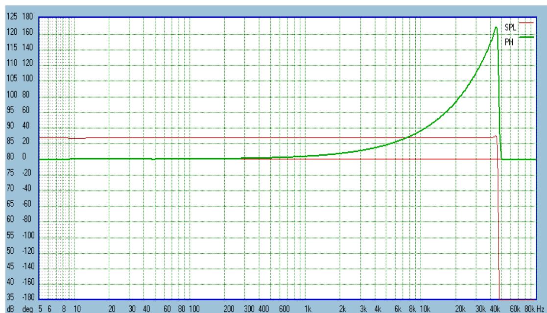
Figure 2. Thick green line shows 10usec tolerance re-calculated as differential phase between the two loudspeakers.
